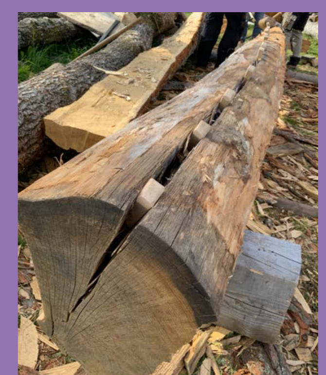
Figure 5. Cleaving perpendicular to grain, from side face of log. Only wooden wedges are used.
