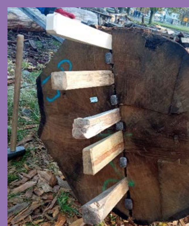
Figure 4. Cleaving parallel to grain, from bottom end of log. Both wood and steel wedges are used.
