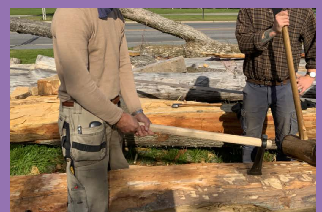
Figure 7. Using the bleggøks to make an incision in the log.
